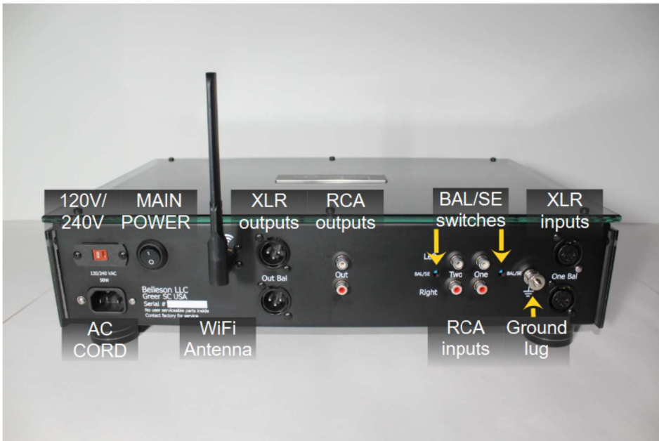
Figure 1: Rear panel connectors and switches
